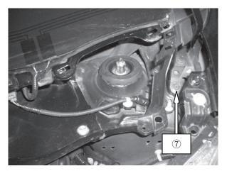
8.) Remove the end brackets from the strut bar and mount them using the included M6 x 20 bolts on the strut tower like pictured.
