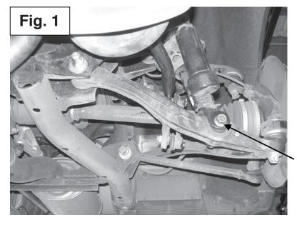
1.) Remove rear lower bolt on the right side of the vehicle.
