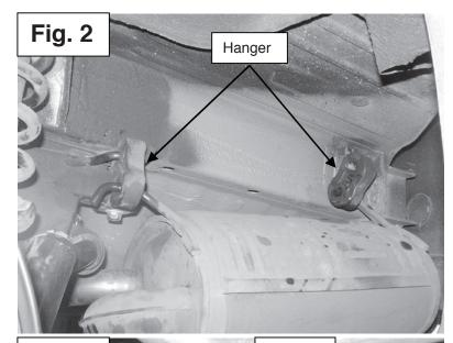
2.) Remove the exhaust hanger rings from both sides. (total 4pcs)
