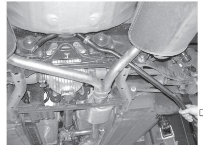
5.) Remove the sway bar from the right side of the vehicle.
