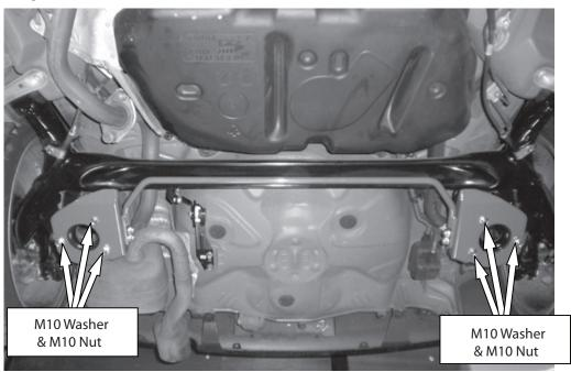
1.) Position the stabilizer bar as shown above and pass through the included M10  $\times$  20 bolts from the spring seat side. Use the included M10 washer and M10 nut on the stabilizer plate side to secure the unit.
