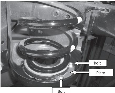
1.) Align the plate bracket on top of the spring seat and install the bolts through the available holes. (Pictured is the driver side, do the same for passenger side)
