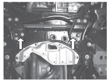
9.) Remove the 4 bolts on both sides to remove the plates. The sway bar may fall so use caution when removing. The sway bar can be pulled out from the left side.
