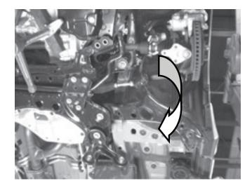
8.) Rotate the lower arm towards the rear of the car. (Use the loosened bolt as a pivot axis)
