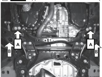
3.) Remove the 4 bolts displayed as "A". Loosen the 2 nuts displayed as "B", three full turns. (Do not completely remove the nuts)
