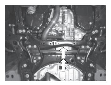
6.) Remove 1 bolt and 4 nuts holding the transmission mount.
