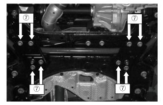
7.) Remove the bolts holding the sway bar brackets. Use caution as the sway bar will drop after all the bolts have been taken off.
