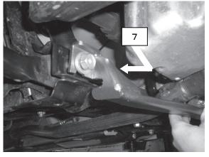
7.) Slide the Powerbrace on to the bolt as pictured, then torque down according to the factory service manual specification.
