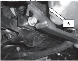
6.) For the driver side (right side), place the Powerbrace between the oil pan and cross member. Further loosen the bolt up to 20mm to enable clearance for the slot to slide in.
