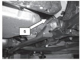
5.) Slide in the Powerbrace horizontally on the passenger side (left side).
