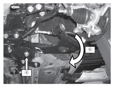
6.) Use the bolt loosened in step #4 as an axis to pivot the lower control arm towards the rear.
