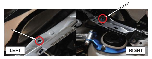
8.) Make sure that the holes are aligned on the strut tower bracket to the metal cowl when installing.
