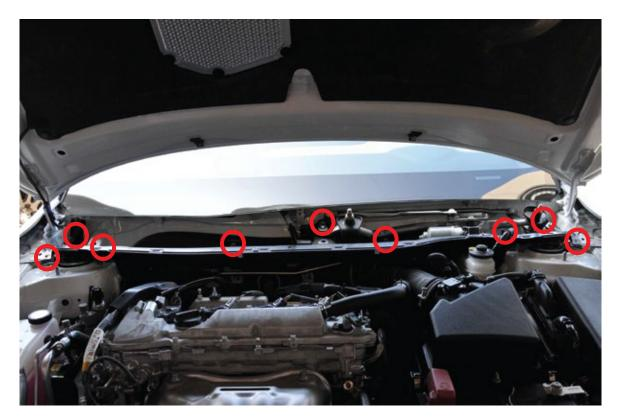
6.) Remove nine 10mm bolts to completely take off the large metal shielding cowl.
