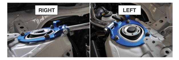
7.) Place the included three washers on each side of the studs on the strut tower. Install strut bracket ends onto strut towers as shown. Do not install the center bar yet. Torque down six nuts that are included with the kit to 50 N.m. (510 kgf.cm, 37ft.lbs)
