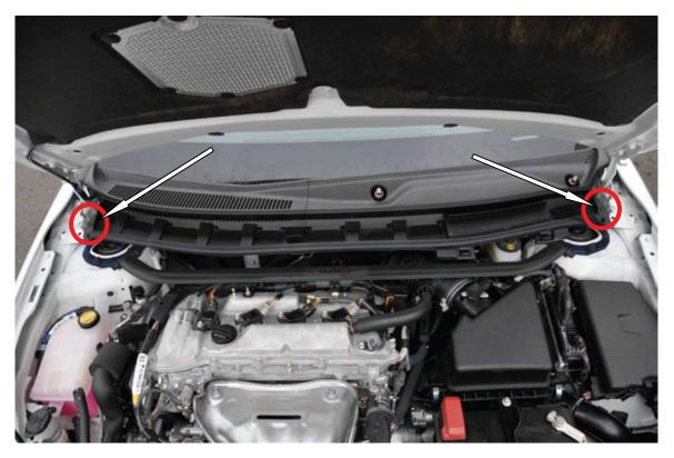
3.) Remove two plastic clips located on the left and right corners of the plastic cowl. Pop in the center dowel first to easily pull off the clip. Carefully remove entire plastic cowl tray from vehicle, exposing the wiper motor assembly
