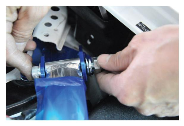
8.) Install the main bar with the washers and crush washer in this order. Hand tighten both ends, then torque down with a 17mm wrench and hex allen head driver.
