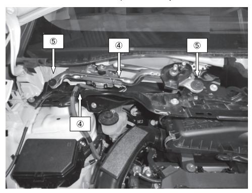
6.) Take off all the bolts indicated below to remove both left and right metal cowl top assembly.
