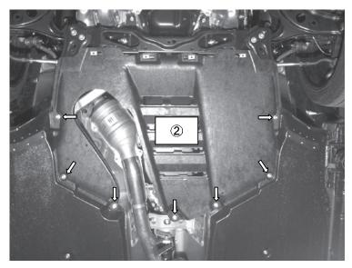
2.) Remove the rest of the undertray by taking off the bolts indicated with the arrows.
