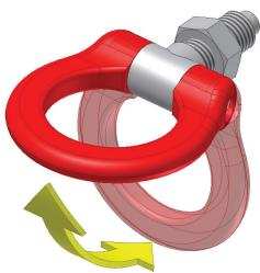
• Make sure the ring is screwed in to the adapter shaft with more than 20mm of threading.
