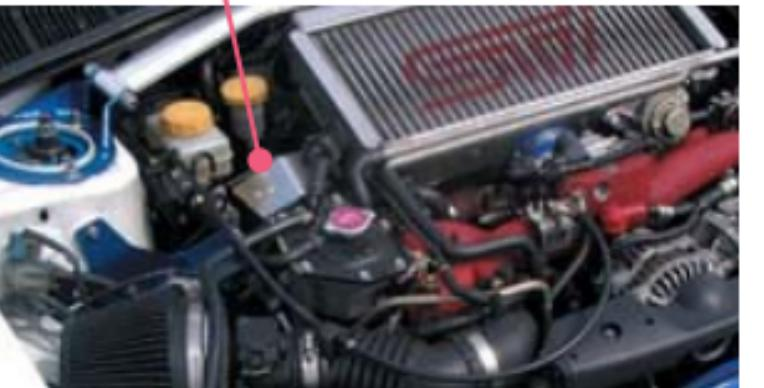
Impreza Turbocharger heat shield
