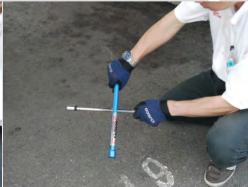
Assemble wrench in cross pattern
