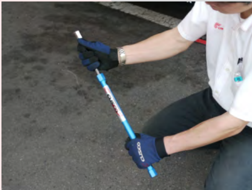
Slide the inner shaft out from blue sleeve
