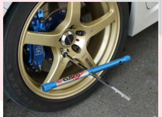
Slide shaft into outer most hole for more torque
