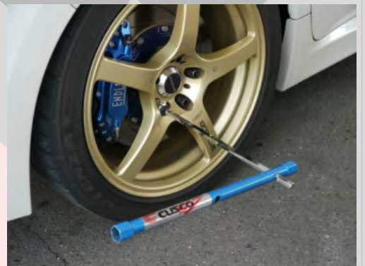
Slide shaft into outer most hole for more torque
