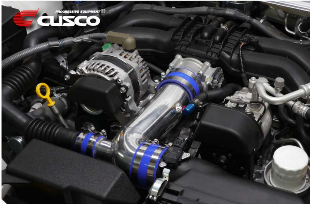
Air Suction Pipe Kit installed with sound creator option intact
