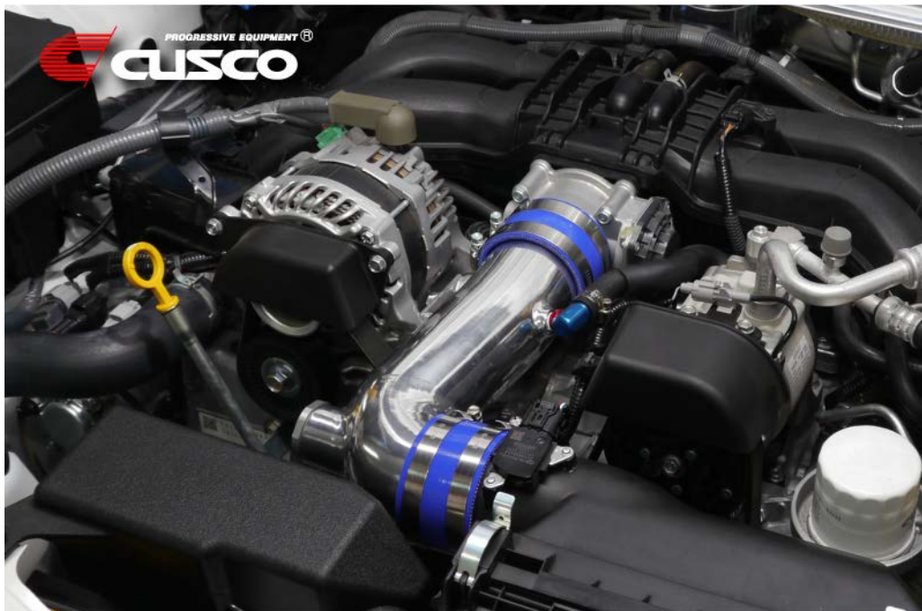
Air Suction Pipe Kit installed with deleted sound creator option
