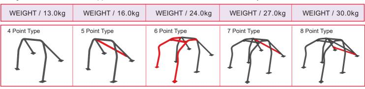
5 Point Type A diagonal pipe added to the 4 Point Type
