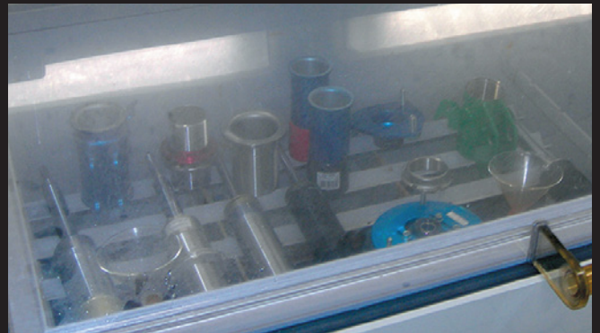
High concentration saltwater direct injection test
