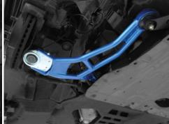
Not Applicable at  $\pm 15$ mm position when using OEM tie rod end. Make sure there is more than 20 mm for screws to contact at tie rod ends.
