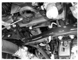
Slide the sway bar to left, careful not to touch air conditioning pipes.
