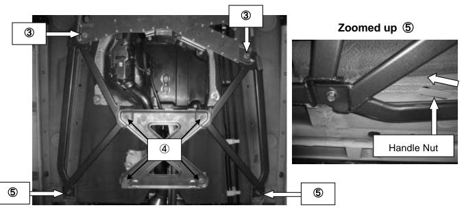
%Above picture shows installation with 429 492 R(Rear Power Brace).
