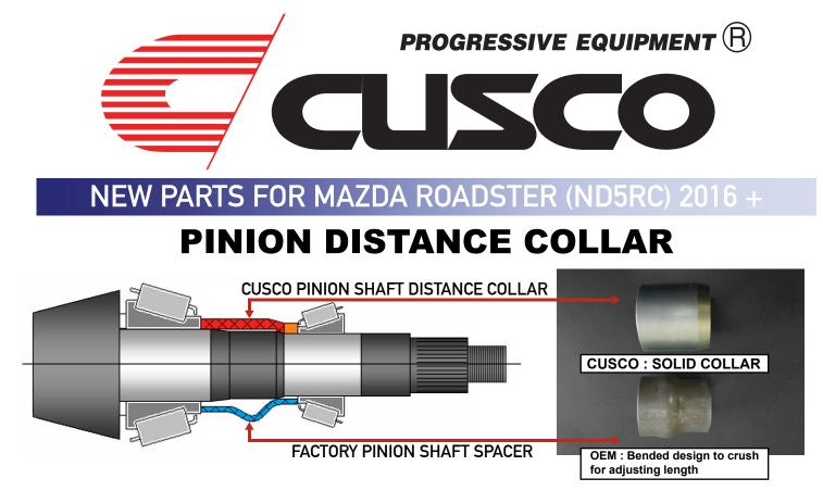
The Cusco Pinion Distance Collar is made more solid and designed to withstand the abuse of constant acceleration and deceleration, and is recommended for vehicles putting out more power & torque than the factory output.
