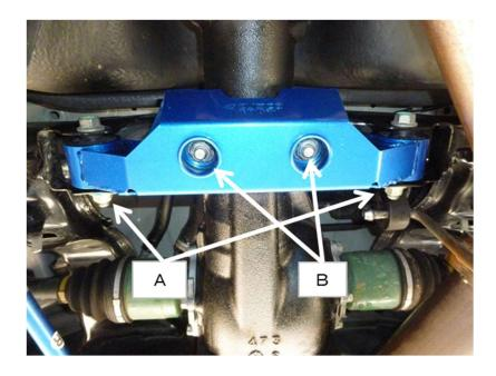
Tightening Torque: A 110 N-m / 81 ft-lbs B 50 N-m / 37 ft-lbs.
