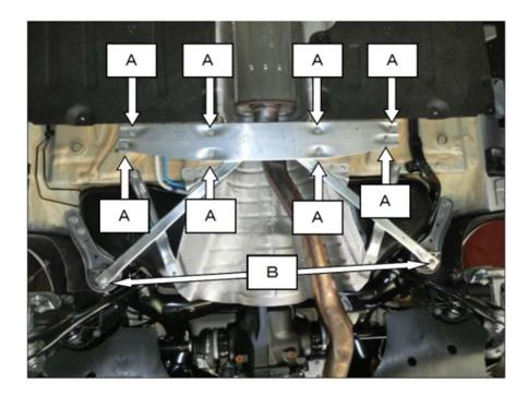
Torque Spec: "A" Bolt (x8): 26 Nm/19 ft-lbs. / "B" Bolt: 56 Nm/41 ft-lbs.
