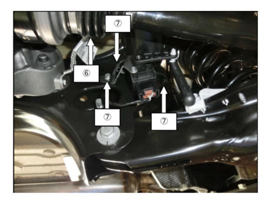
8. Remove x2 harnesses (to Brake Caliper) and hoses (#8) for free moving.
