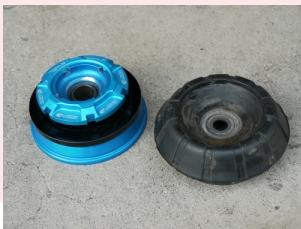
Left: Cusco Centerlock Right: Factory upper mount
