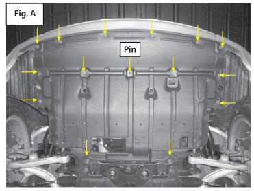
1.) Remove the 14 bolts + 1 pin shown in Fig. A to take off the undercover tray.
