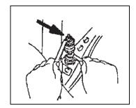
3.) To remove the tension rod assembly, do not part the rod from its bracket, but remove the entire bracket with the tension rod still in place.
