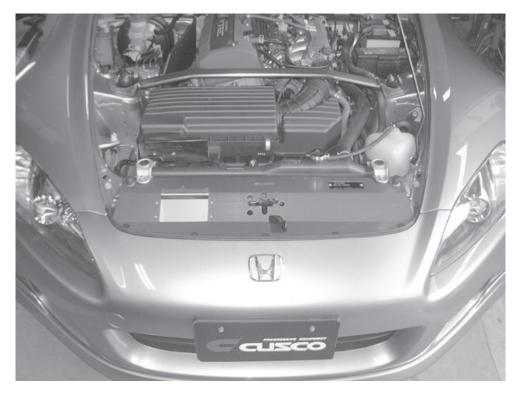
3.) Place the cooling plate as shown in the photo above and reinstall the two radiator support brackets on top of the cooling plate. The five weather stripping bolts will also be reused.
