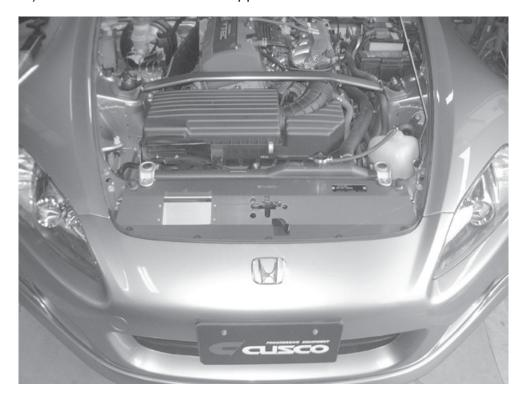
3.) Place the cooling plate as shown in the photo above and reinstall the two radiator support brackets on top of the cooling plate. The five weather stripping bolts will also be reused.
